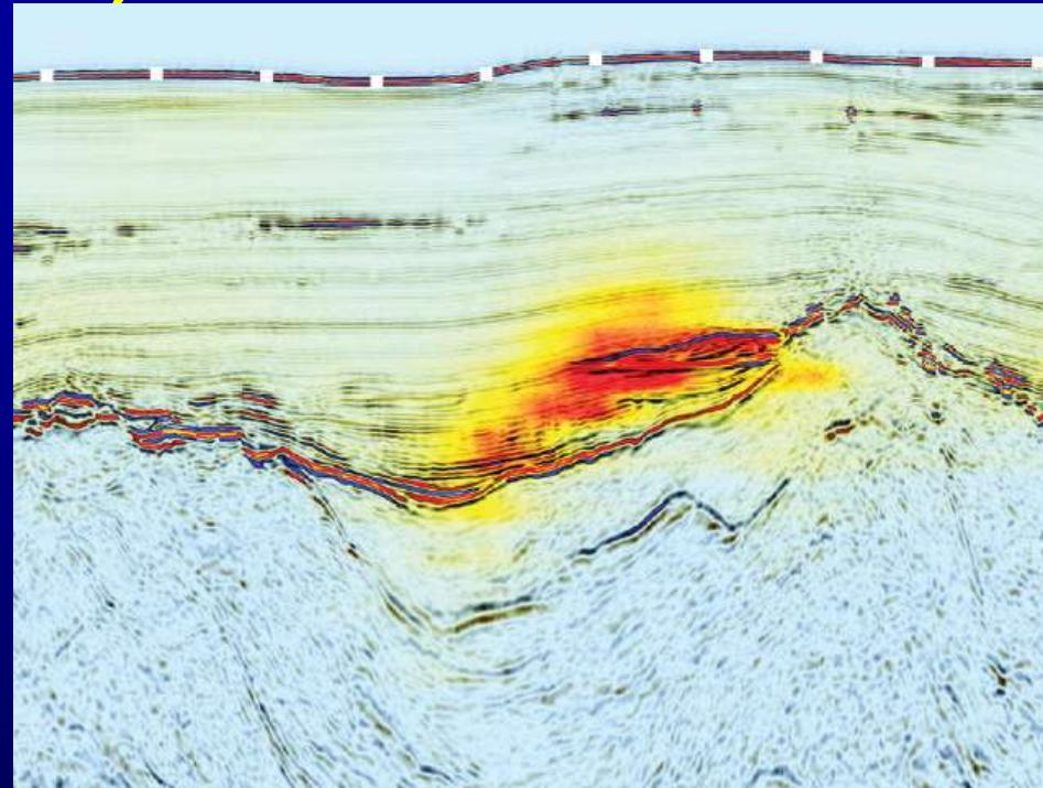
Figure 2: EM-imaging data integrated with seismic data shows which of the structures identified on a seismic image is likely to contain hydrocarbons and which can be discounted from further geophysical or drilling investigations. EM surveys measure resistivity; hydrocarbon-charged reservoirs typically have a much higher resistivity than the surrounding rock, as indicated by the red colour in the image above. (Data courtesy of Murphy Oil Corporation.)
