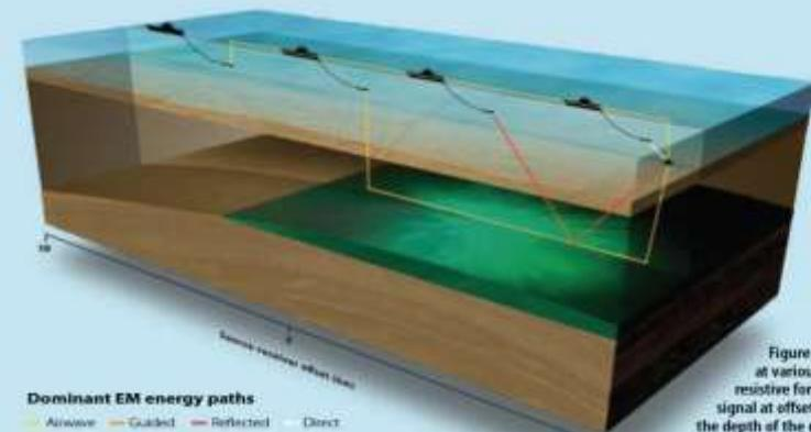
Figure 4: The path of the dominant energy at various offsets is shown. Energy guided by resistive formation layers dominates the received signal at offsets typically greater than three times the depth of the guiding layer (yellow).
